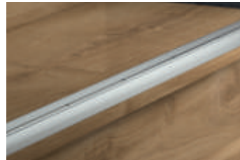
5 Stair nose aluminium (on request) Fits to flooring thickness of 7 - 16 mm, W = 23 mm, L = 2.7 m. PGSTPSILV, silver. Surface: aluminium.
